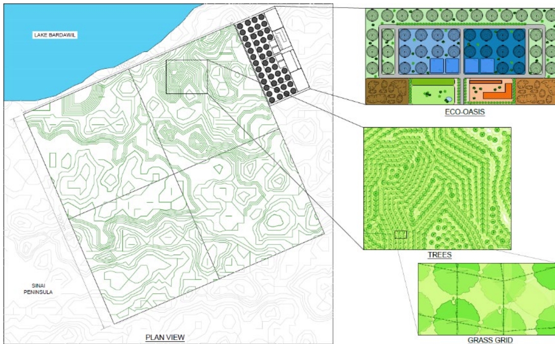
Figure 1-4. Plan view of the 1 km 2 regreening site and adjacent Eco Oasis ® . The close up of the grass grid, are (dried) salt tolerant grasses grown in the second stage of the revitalizing section (see Figure 1-5 below).
